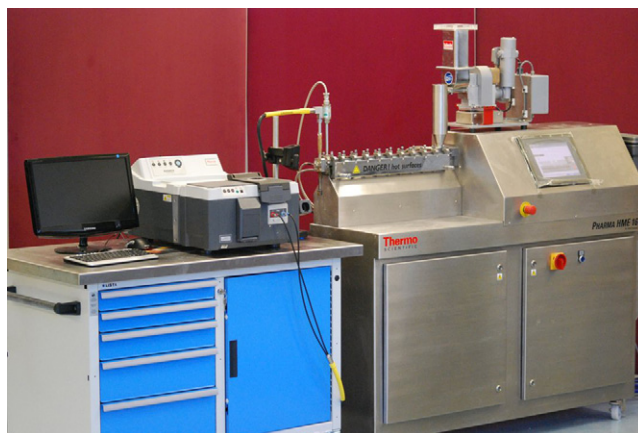
Fig. 1. Pharmalab HME16 extruder equipped with NIR probe connected to the Antaris II NIR spectrometer.
